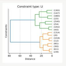
Dendrograms showing agglomerative clustering by constraint features. The x-axis shows the Euclidean distance between clusters. On the y-axis labels indicate the number of data points in a branch.
