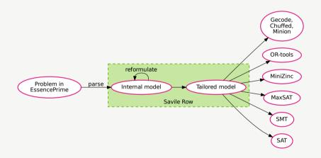
Using Savile Row to reformulate and solve CSPs using various back-end solvers
